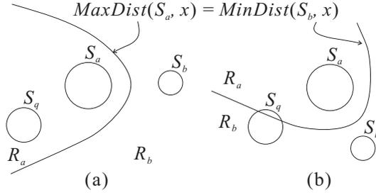
**Figure 6: An example illustrating the Voronoi-based approach**
