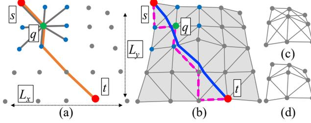
Fig. 2. (a) A point cloud with orange  $\Pi^*(s, t|C)$ , (b) a *TIN* with blue  $\Pi^*(s, t|T)$  and pink  $\Pi_N(s, t|T)$ , (c) a conceptual graph of a point cloud, and (d) a conceptual graph of a *TIN*
